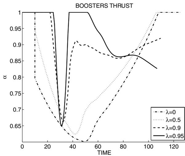
Fig. 5 Regularization homotopy: thrust level for  $\lambda = 0, 0.5, 0.9$ , and  $0.95$ .
