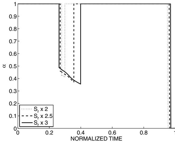
Fig. 7 Singular arcs for increasing values of  $S_r$ .
