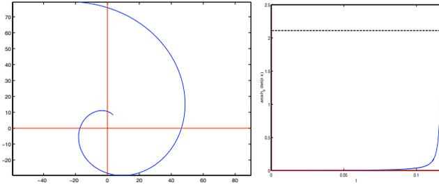
Fig. 2. An exceptional trajectory. The initial cumulated longitude  $l_0$  is in  $]0, \pi[$ ,  $l_0 = 3\pi/8$ , and the satellite spirals up so that  $|q| \rightarrow \infty$ , leaving rapidly the elliptic domain. The associated determinant remains negative, ensuring  $\mathcal{C}^0$ -local optimality of the whole trajectory.
