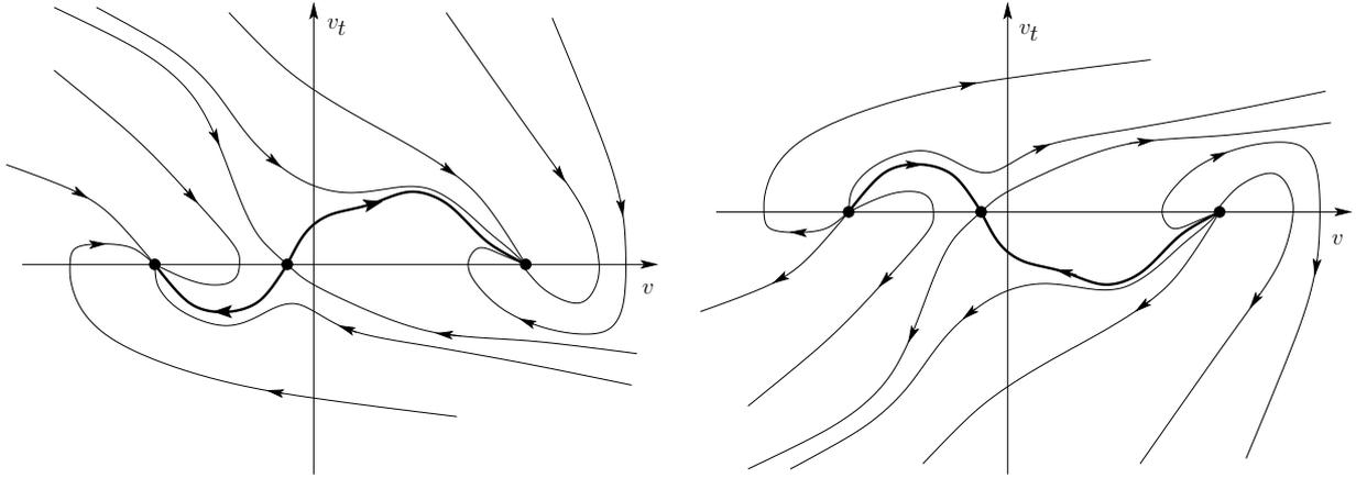
Figure 1: *Right: the flow of the dynamical system  $S(t)$  generated by the feedback control  $u = \gamma(x)v_t$ . The flow is represented in the phase plane  $(v, v_t)$ . The compact global attractor  $\mathcal{A}$  (in bold) consists in three equilibrium points and two heteroclinic orbits connecting them. Left: the flow generated by the feedback control  $u = -\gamma(x)v_t$ . It is deduced from the flow of  $S(t)$  by reversing time and orientation of the second coordinate.*
