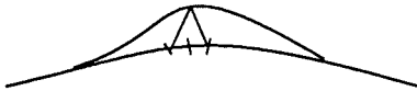
Figure 5 Sketch of a CAD-free deformation without and with the regularization operator. The initial deformation is only C^0(\Gamma) and to have a C^1(\Gamma) variation, one needs to project it, for instance, into H^{5/2}(\Gamma) if \Gamma is a surface in \mathbb{R}^3 .
