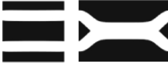
Figure 3 Borwall & Petersson solved the problem of the cheapest (drag) transmission of fluid from left to right for a given volume of pipe. Topological optimization was used so as to handle topological changes such as seen here between the initial guess and the computed solution (Borwall et al. 2001).
