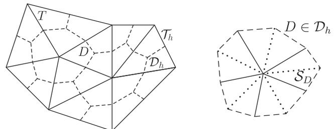
Fig. 1. Simplicial mesh  $\mathcal{T}_h$  and the associated vertex-centered dual mesh  $\mathcal{D}_h$  (left) and the fine simplicial mesh  $\mathcal{S}_D$  of  $D \in \mathcal{D}_h$  (right).
