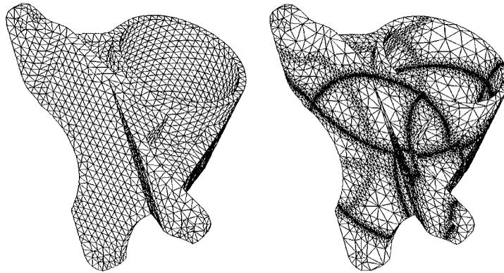
Figure 14. Adapted surface mesh, iterations 0 and 3
