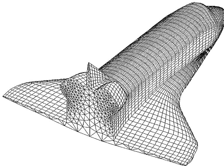
Figure 12. Surface triangulation of the Columbia shuttle
