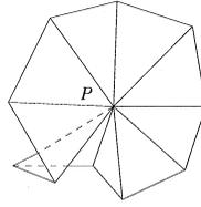
Figure 1. Vertex  $P$  is a non-conforming vertex
