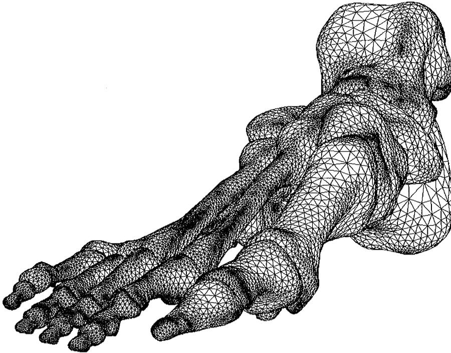
Figure 9. Optimized surface triangulation of a foot skeleton
