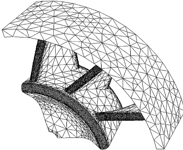
Figure 13. Optimized mesh of a mechanical device
