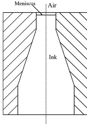
**Figure 5** The cross-section view of an inkjet nozzle.
