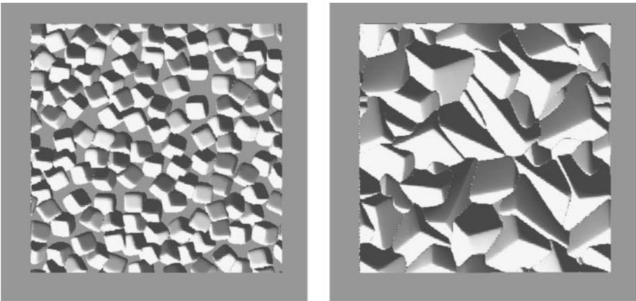
**Figure 8** The growth of a diamond film. Here, the diamond grows with a cubic structure. The figure on the *left* is at an early time, whereas the figure on the *right* is at a later time. From P. Smereka, X. Li, G. Russo, & D.J. Srolovitz (manuscript in preparation).
