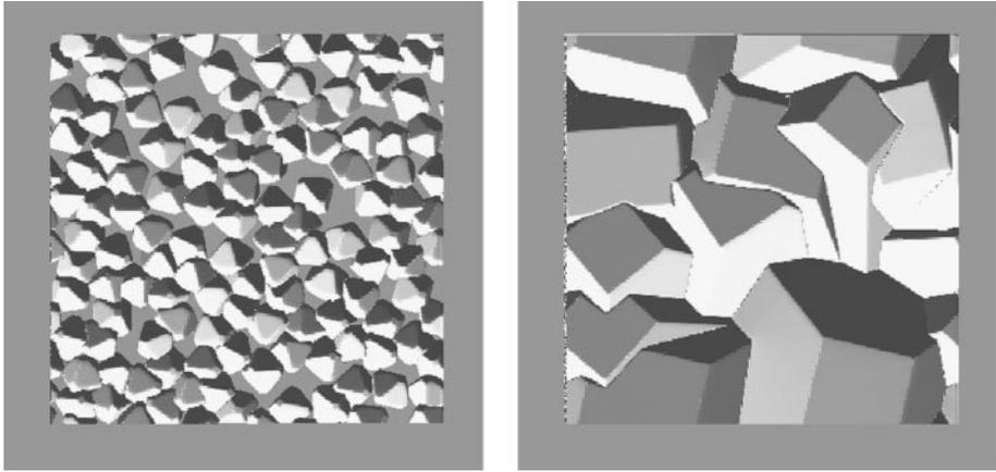
**Figure 9** The growth of a diamond film. Here, the diamond grows as a 14-sided polyhedron. The figure on the *left* is at an early time, whereas the figure on the *right* is at a later time. From P. Smereka, X. Li, G. Russo, & D.J. Srolovitz (manuscript in preparation).
