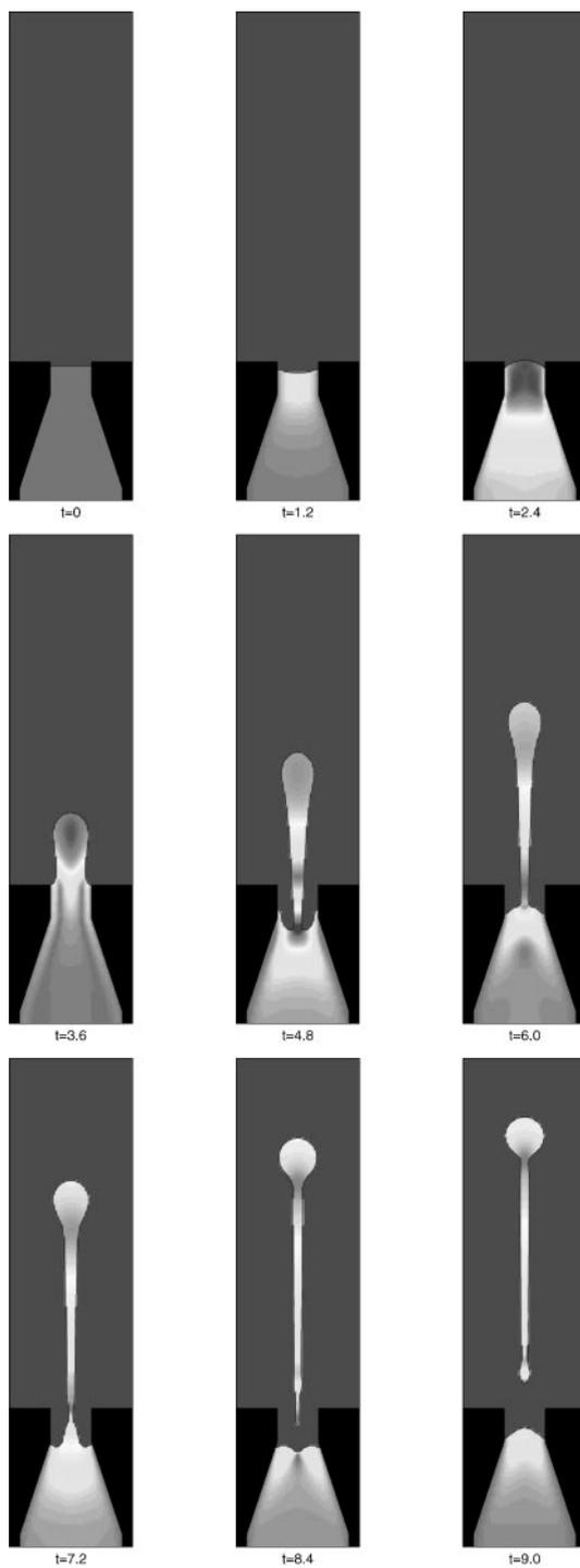
**Figure 7** Ejection of an ink droplet.
