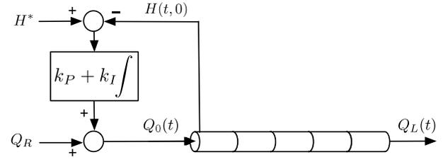
Fig. 2. Block diagram of the closed-loop system with a Proportional–Integral control.
