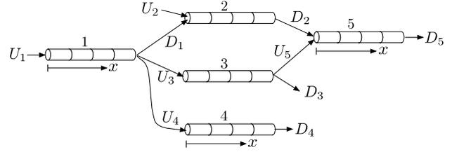
**Fig. 3.** Physical network of density-flow systems.
