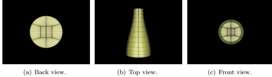
Fig. 18. Pipe with scaled cross-sections,  $\Phi_s$ .
